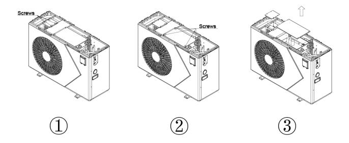
Step 4: Remove the front panel
