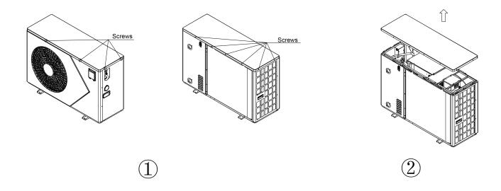
Step 3: Remove the electrical box cover
